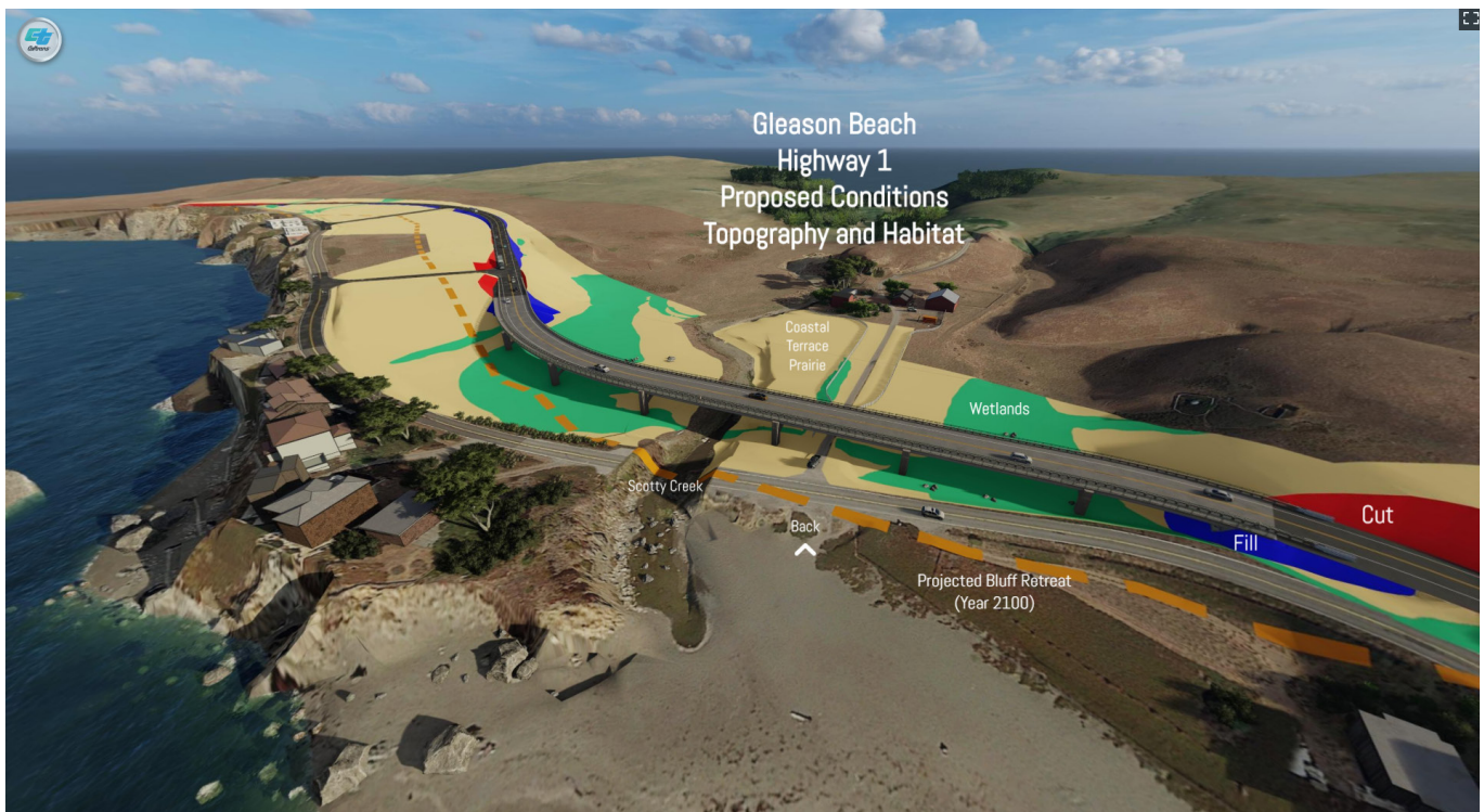
Aerial View of Topography, Habitat, Projected Bluff Erosion, and Proposed Highway Realignment
