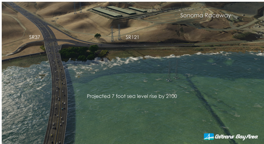
Proposed Elevated Highway over Projected Sea Level Rise
